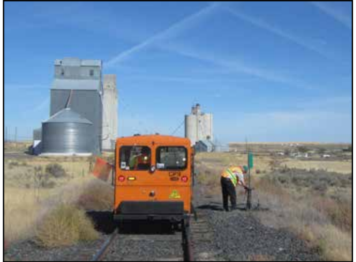
Anticipating the arrival of an afternoon freight train, the railroad pilot throws the switch stand to put the group into Govan siding.
