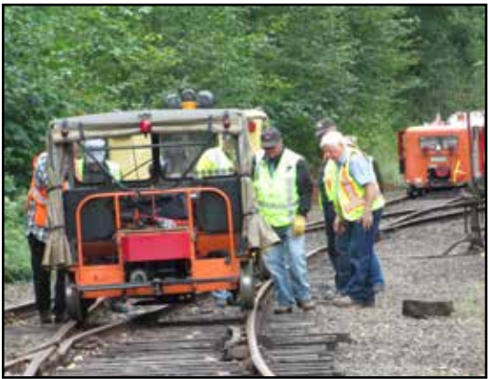
Preparing to depart Chelatchie, the group encountered a wide gauge turnout. Volunteers pushed motorcars by hand over the troublesome spot.
