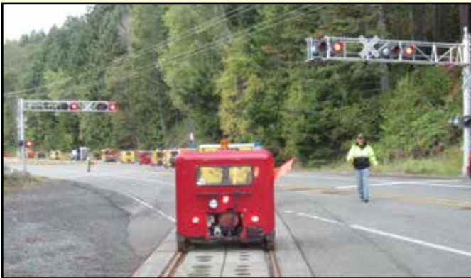
Leaving Elbe, the signals were shunted to protect the motorcars crossing the National Park Highway.
