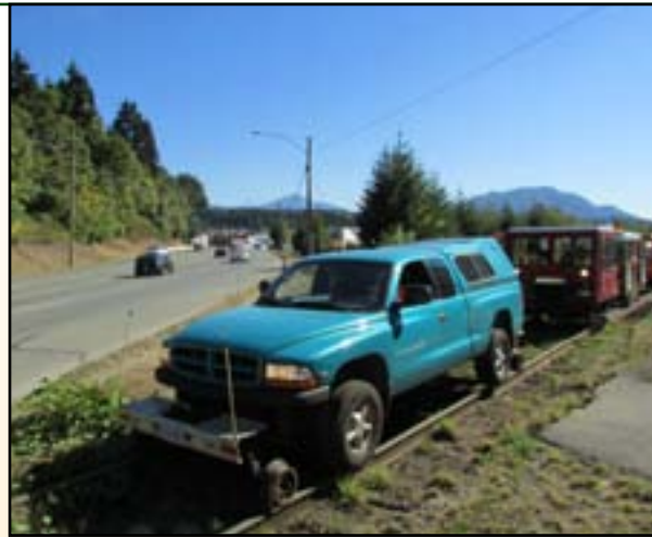
Hi-rail truck and motorcars hold at busy Stamp Avenue for the flagging team to come forward on the way out of Port Alberni.
