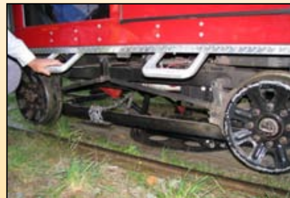
It was determined the rear torsion arm broke loose from the motorcar frame. The broken member was then chained to the frame to continue the trip to Parksville.
