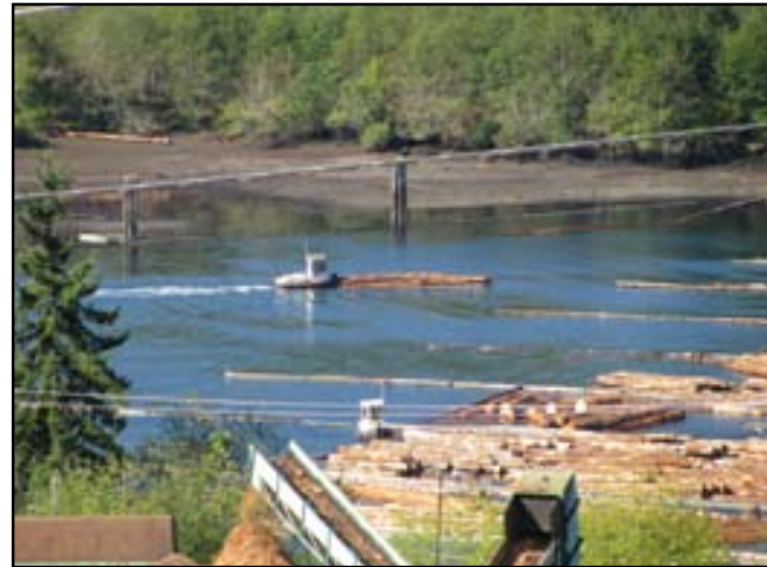
A tugboat assembled timber rafts at Beaver Cove. Logs are bundled into timber rafts for floating the logs across the Johnson Strait to the British Columbia mainland lumber mills.
