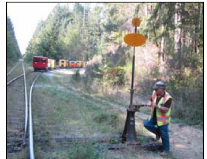
John Haverty throwing the McLean Mill switch, returning the motorcars to the mainline.
