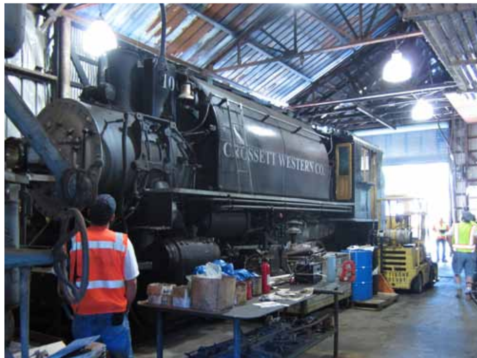
Right: Members had the opportunity to visit the Chelatchie locomotive shop and view the Crossett Western Lumber Company Alco 2-8-2 tank locomotive. The all volunteer Chelatchie Prairie Railroad recently purchased the engine for their special events.
