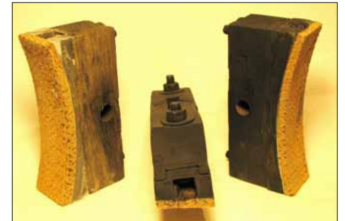
The liner's edges and lining on the left have been dressed while on the right the liner has been spray painted in preparation for installation. Observe the center liner's end. Its taper conforms to the wheel tread and no break-in period is necessary.
