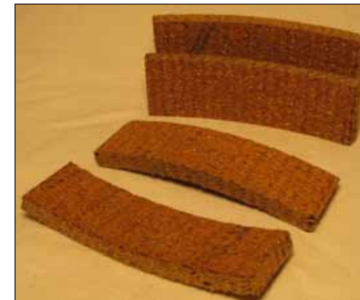
The four FRAS-LE woven brake linings prepared and delivered by the Chester Avenue Brake Company. Note the lining's manufactured curve.
